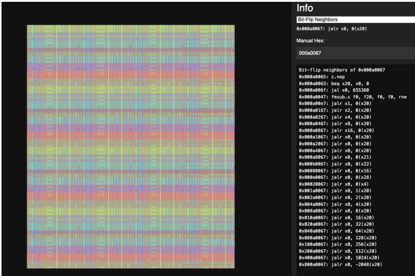
Fig. 7: We generated a visualization that shows all instructions 1 bitflip away from a given instruction. This figure demonstrates the neighbors of jalr x0, 0(x20)
